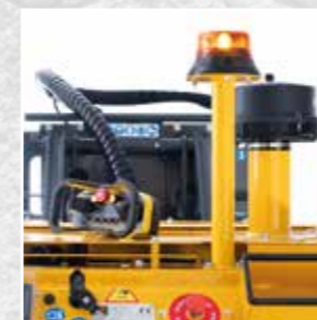
Engine aspiration with prefilter cyclonic for a cleanest combustion air.
