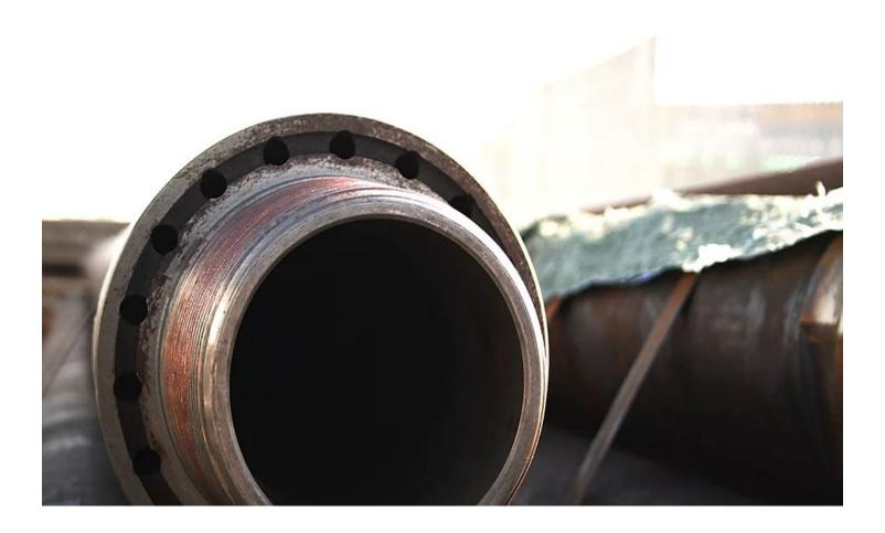
Friction drill pipes for reverse circulation are used in applications where the priority is to recover all debris produced during drilling or when it is necessary to prevent the drilling fluid used to disperse into the subsoil. This type of rod, therefore, has two separate channels for the circulation of drilling fluid. ColliDrill produces rods for reverse circulation with diameters between 90 and 220 mm.
